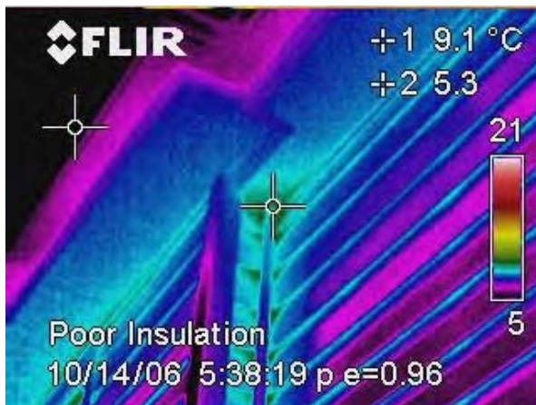
Figure 3. Thermogram and photo pair showing air leakage in a house inspection.
