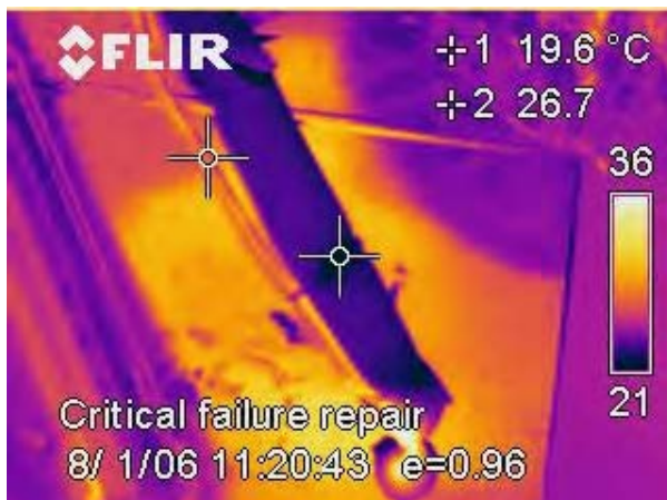
Figure 5. Thermogram and photo pair showing inefficient new A/C system.
